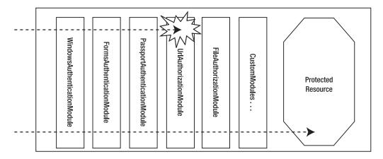
Figure 19-9. The ASP.NET security gatekeepers as IHttpModule classes
