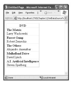
Figure 12-10. XML data binding with templates
