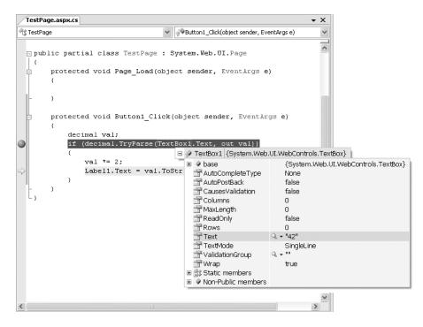
Figure 2-24. Viewing object properties in break mode
