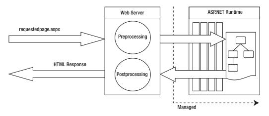
Figure 18-3. High-level ASP.NET architecture
