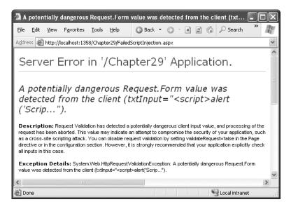
Figure 29-7. A failed script injection attack
