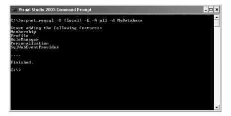
Figure 21-5. Executing aspnet\_regsql.exe for installing the database
